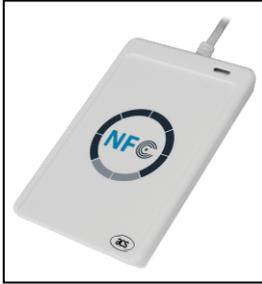
The ACR122U is a PC-linked contactless smart card reader/writer developed on the 13.56 MHz contactless technology. It is the world's first CCID-compliant contactless card reader/writer that follows both ISO 14443 and ISO 18092. This device is designed to support not only Mifare and ISO 14443 Type A and B cards, but also FeliCa and NFC tags.
